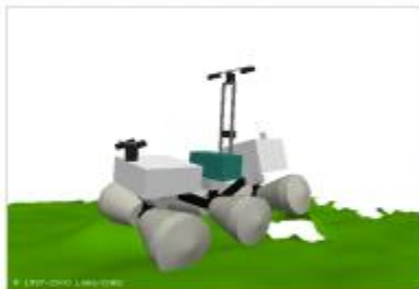
Convolution of the robot Kinematics (only) model with the terrain model
